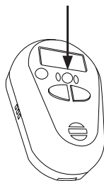
Fig. 1 EN: Test/Silence button, control lamps SV: Test/Silence knapp, kontrollampor DE: Test/Silencetaste, Kontrollleuchte NO: Test/Silenceknapp, kontrolllampe ES: Botón de prueba/silenciar, luz de control
